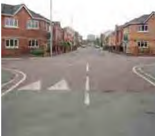
Figure 7.13 Raised tables at junction in Hulme. The table has been raised almost to kerb height.
